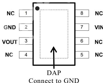
The DAP is used as a thermal connection to remove heat from the device to an external heat-sink in the form of the copper area on the printed circuit board. The DAP is physically connected to backside of the die, but is not internally connected to device ground. The DAP should be soldered to the Ground Plane copper.
