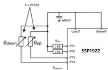
SSP1922 also supports the measurement of PT100 sensor, but the measurement stability will be reduced. In THIS CASE, WE RECOMMEND CONNECTING BOTH REFERENCE resist ORS RATHER THAN JUST ONE. As shown on the right. This will help to compensate the gain offset of the temperature sensor in the whole temperature range by the two point temperature accuracy.
