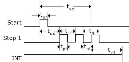
Each input separately can be set to be sensitive to rising or falling edge. This is done in register 0, bits 0 to 2. (NEG\_START, NEG\_STOP1). Further all Start/Stop-inputs support a high active enable pin.
