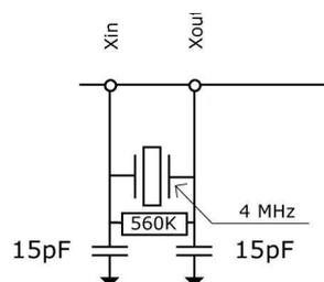
The programmable delay guarantees that the oscillator has settled before the measurement starts. For ceramic resonators 480  $\mu\text{s}$  will be sufficient. By this measure the average current consumption can be drastically reduced.
