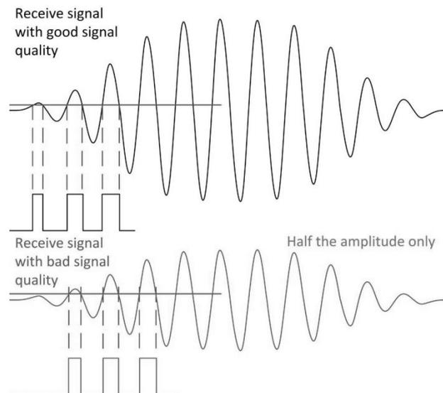
With the SSP1922's first wave detection the time-of-flight measurement is related to the first wave and gets independent from temperature and flow. Miscalculations due to wrong zero crossing assignment are no longer possible.
