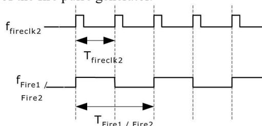
As shown in Figure above at least 2 clock periods  $T_{\text{fireclk2}}$  are required to send one fire pulse. One for the high
