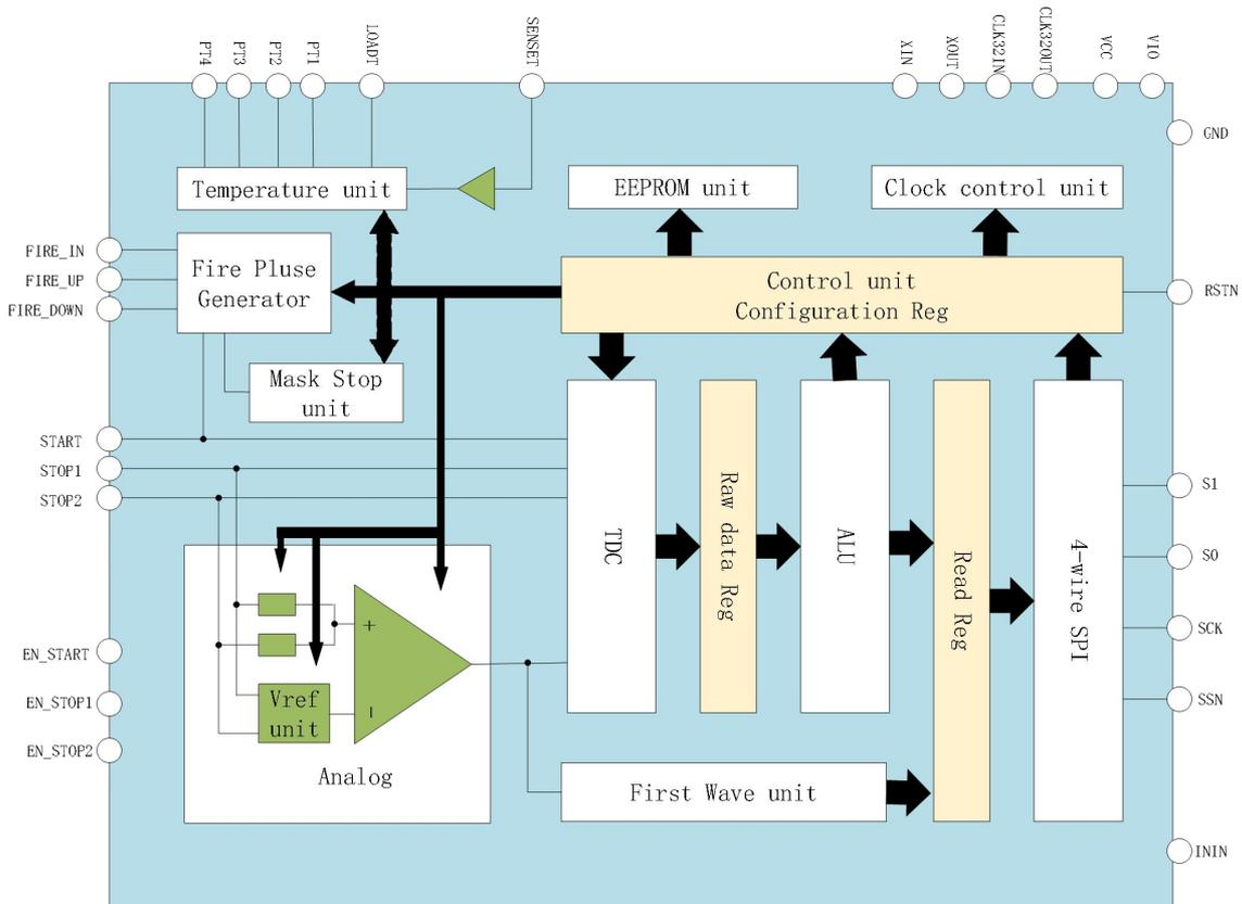
Figure 1 Block Diagram
