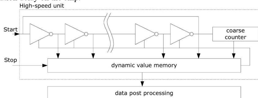
The measuring unit is triggered by a START signal and stopped by a STOP signal. Based on the position of the ring oscillator and the coarse counter the time interval between START and STOP is calculated with a 20 bit
