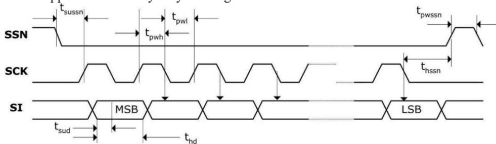
Figure 3 SPI Write
