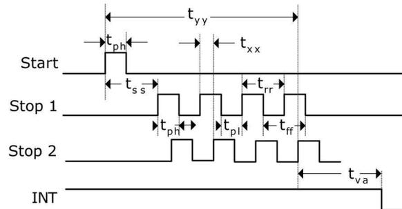
Each input separately can be set to be sensitive to rising or falling edge or both edges. This is done in register 0, bits 8 to 10. (NEG\_START, NEG\_STOP1, NEG\_STOP2) and register 2, bit 27 & 28, RFEDGE. Furthermore all Start/Stop-inputs support a high active enable pin.
