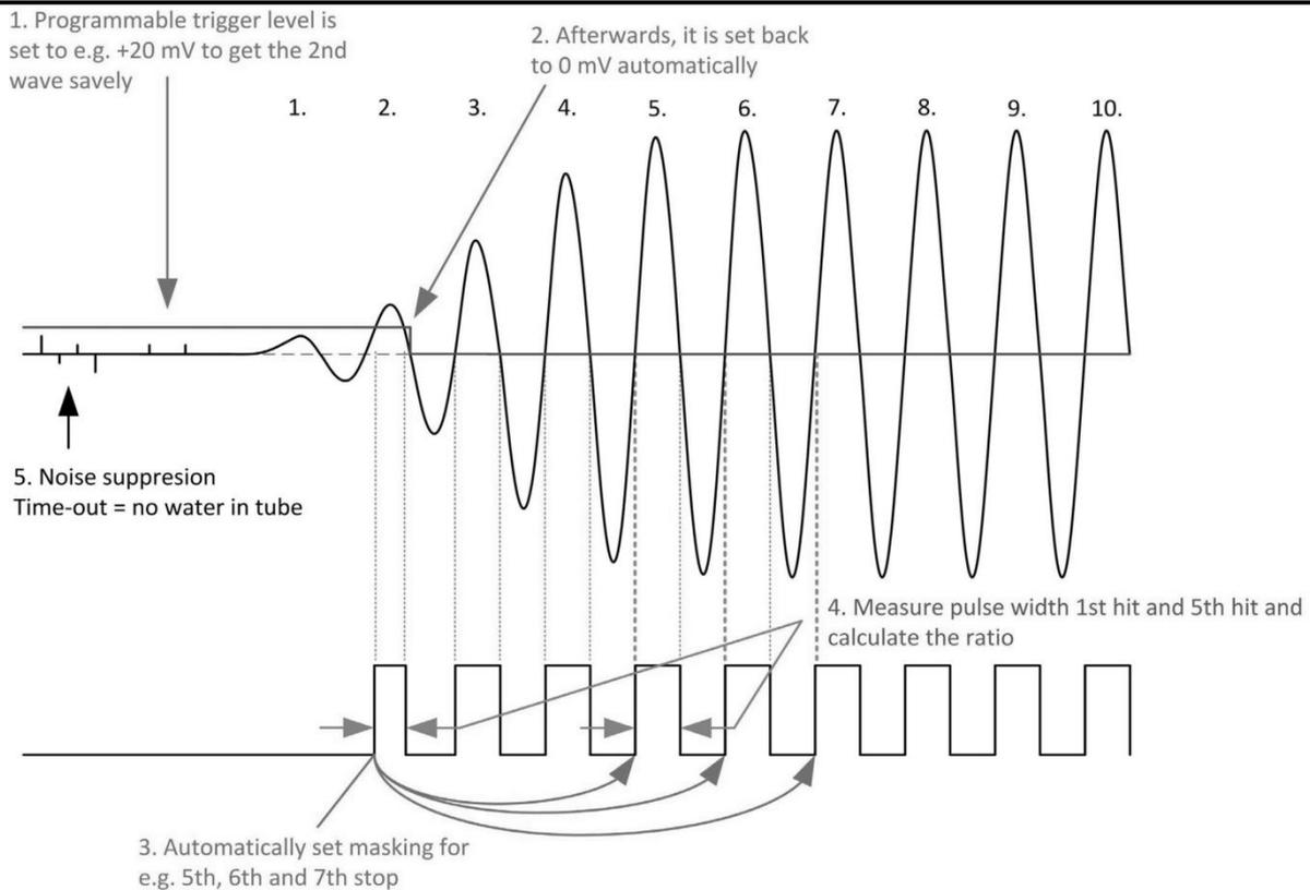
1. With the fire pulse generator the offset for the first wave detection is set to a programmable level. The DELVAL1 stop masking is used for surprising any noise and it is set just roughly close to the minimum expected time-of-flight. Further noise will be suppressed by the comparator offset until the receive signal reaches the amplitude above this offset level.
