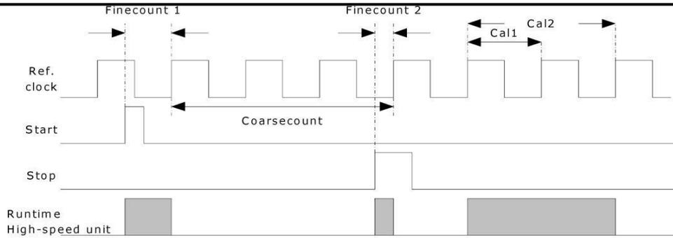
$$\text{time} = T_{\text{ref}} \times (C_c + (F_c1 - F_c2) / (Cal2 - Cal1))$$
