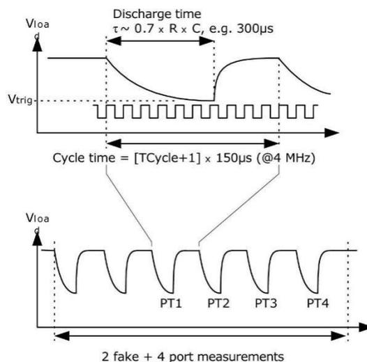
The unit has 4 resistor ports, two of them to be used for the temperature sensors for hot water (up) and cold water (down). The other two ports are used for reference resistors. Basically, on reference resistor connected to both ports is sufficient.
