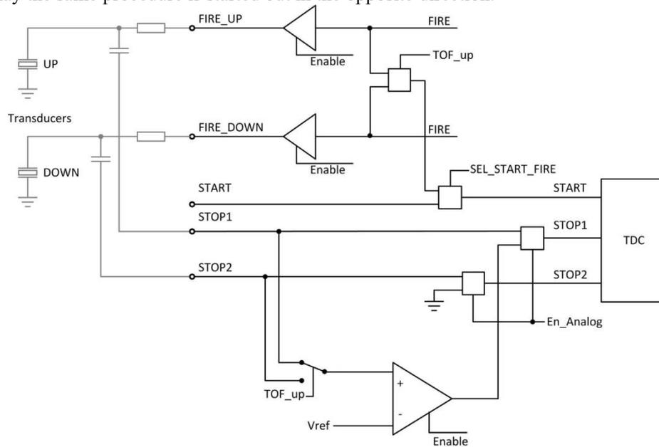
The offset of the comparator can be set in steps of 1mV from -8mV to +7mV by means of parameter DA\_KORR, bits 25 to 28 in register 6. DA\_KORR is set as 2's complement.
