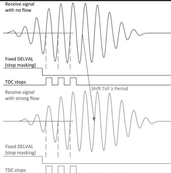
There is still another source of getting wrong measurements. Dirt deposition on the transducers, spool piece mirrors and housing will lead to signal damping e.g. from  $\pm 400\text{mV}$  to  $< \pm 80\text{mV}$ . The figure below shows how this will affect the first wave detection at a given, fixed offset for the first wave detection. Once the first wave amplitude is below the offset level the measurement result will jump by one period.
