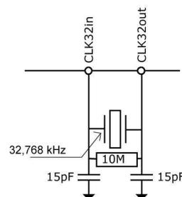
The settling time of this oscillator is about 3 s after power-up. The 32.768 kHz oscillator cannot be switched off.
