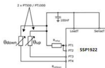
The temperature measurement is fully automated. It is triggered by the  $\mu$ C sending the opcodes Start\_Temp or Start\_Temp\_Restart. With Start\_Temp\_Restart the SSP1922 measures the temperature twice, with a delay given in multiples of the 50 Hz/60 Hz period. This will be of help to reduce 50Hz/60Hz noise.
